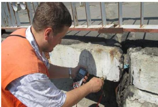
Fig. 1. Measurement of potentials at the site
