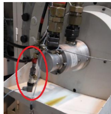
Fig. 1.6. Connection of pressure sensor to C-B unit
