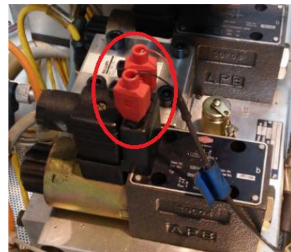
Fig. 1.5. Connection to the coil of PSV
