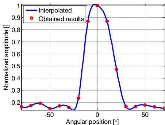
Fig. 17. Measured T-IDT angular sensitivity and its interpolation.
