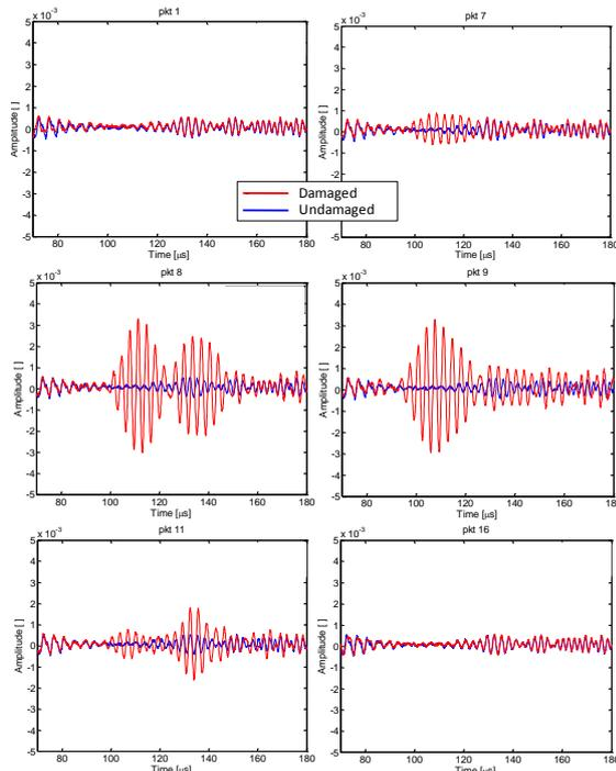
Fig. 16. Exemplary T-IDT measurements for different pad localisations at the excitation frequency of 300kHz
