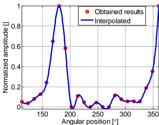
Fig.18. Measured IDT's angular sensitivity and its interpolation
