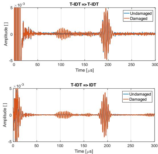
Fig. 14. Exemplary results of experimental tests in different emitter-sensor configuration at excitation frequency of 300 kHz
