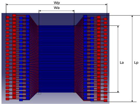
Fig. 3. T-IDT design of the prototype
