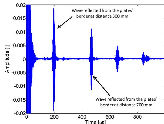
Fig. 10. The T-IDT measurements of the wave reflected from the borders of the aluminium plate at the excitation frequency of 300kHz
