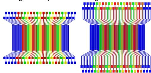
Fig. 13. Configurations of the designed T-IDT for experimental tests; a.) top electrodes b.) bottom electrodes
