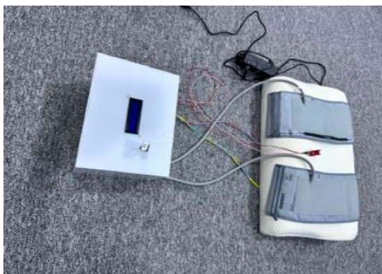
Fig. 3. The optimized design of the pillow
