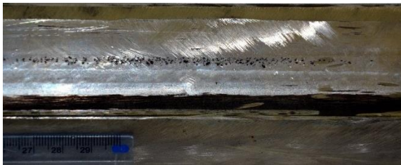
Fig. 12. Section of tooth (260...360 mm) with traces of continued chipping (side B)
