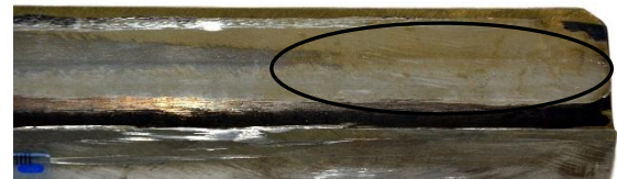
Fig. 9. A loaded section of a tooth with traces of burrs (side A)
