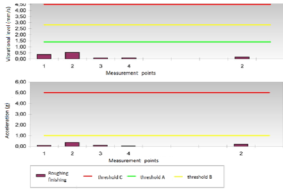
Fig. 4. Velocity and the accelerations measuring on grinding machine vs ISO value
