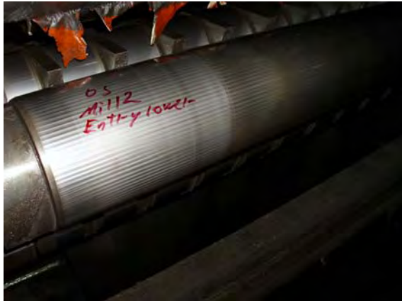
Fig. 2. Chatter marks on the roll
