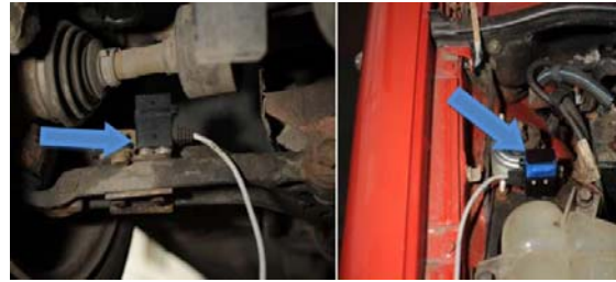
Fig. 10. Arrangement of vibration acceleration sensors
