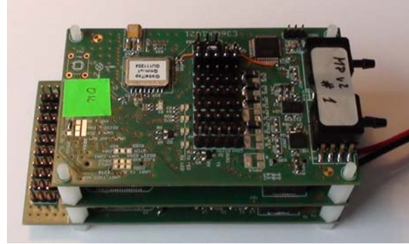
Fig. 2. Integrated AHRS+GPS+ADC module
