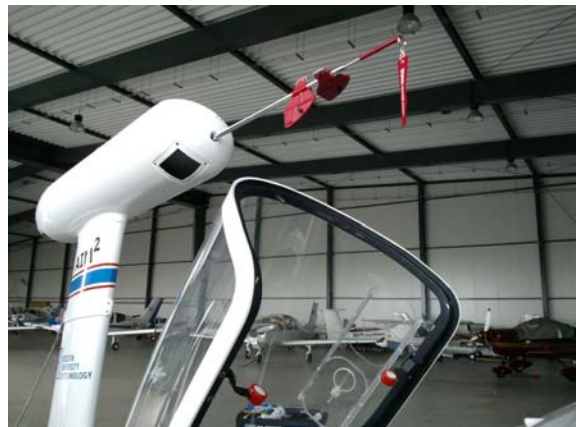
Fig. 11. Aerodynamic probe (with red plugs)
