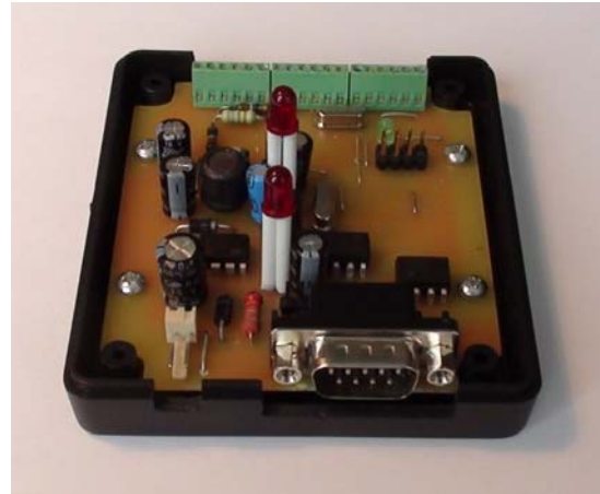
Fig. 5. A/D and digital inputs unit
