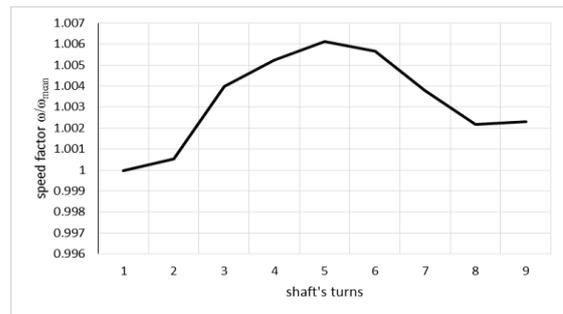
Fig. 7. Mean values of speed factor referring to subsequent shaft revolutions recorded during sea waving (9 revolutions)
