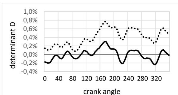
Fig. 6. comparison of determinant  $D$  for healthy engine working at calm sea (solid line) and rough sea (dotted line)
