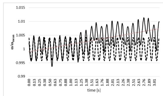
Fig. 4. Comparison of modelled function of speed factor (dotted line) and function of speed factor recorded on real object at waving sea (solid line)
