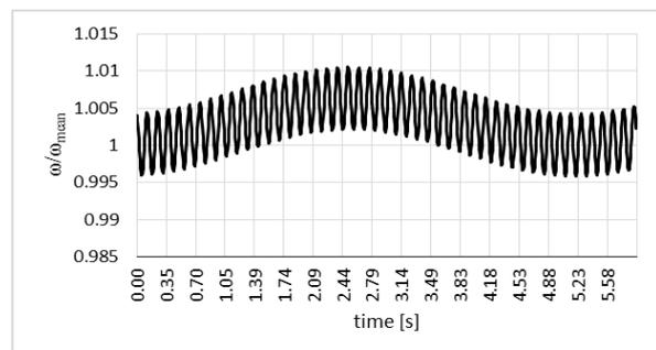
Fig. 8. Model course of speed factor of an engine working at wavering sea
