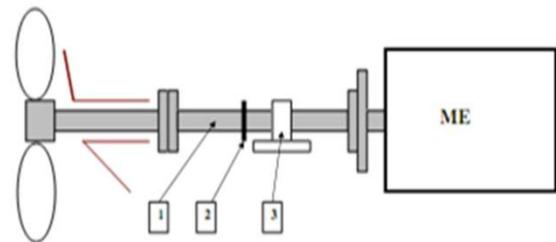
Fig. 2. Scheme of ship's shafting arrangement
