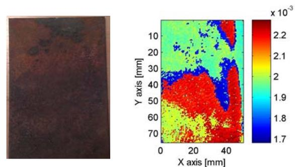
Fig. 4. Corroded plate (left) and the TOF C-scan in mm (right)
