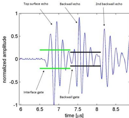
Fig. 2. A-scan with gates
