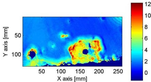
Fig. 6. Corrosion under paint - mapped in dB
