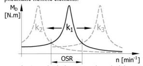
Fig. 1. Mechanical system tuning principle
