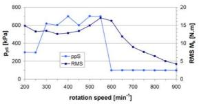
Fig. 6. Optimal air overpressure  $p_{pS}$  and RMS  $M_k$  value in relation to the rotation speed of mechanical system
