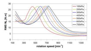
Fig. 3. Resonant curves of the mechanical system at various air overpressure in the tuner  $p_{pS}$
