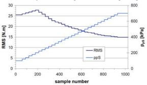
Fig. 7. Example of searching a local minimum of objective function of the mechanical system by the electronic extremal control system MESLER at mechanical system rotation speed *500 min*<sup>-1</sup>
