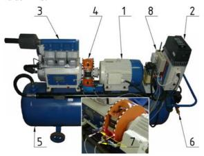
Fig. 2. Implemented torsional oscillating mechanical system
