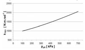
Fig. 4. Dynamic torsional stiffness of the tuner  $k_{dyn}$  dependent on overpressure  $p_{DS}$  in the tuner
