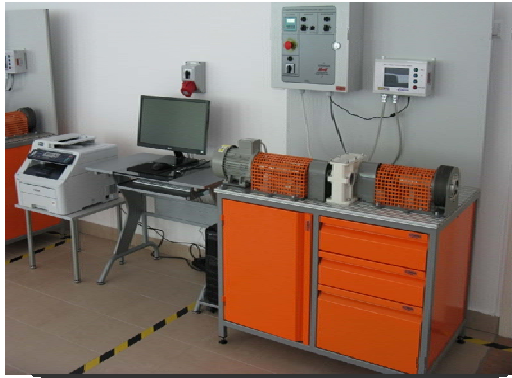
Figure 1 The test stand for testing air gears [1]
