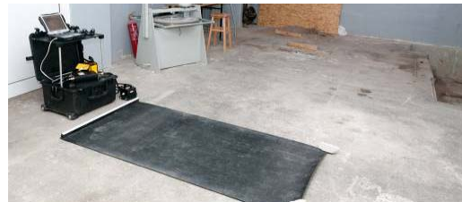
Fig. 4. Ground floor structure during GPR surveys
