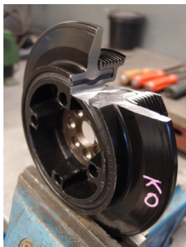
Fig. 2. Torsional vibration damper: a - model of damper, b - a real damper
