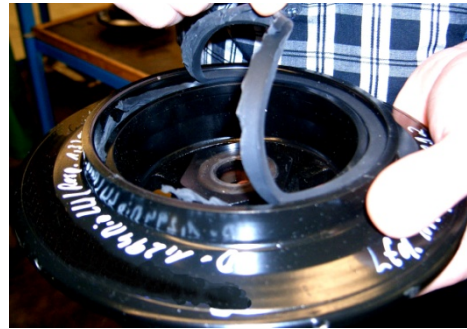
Fig. 3. View of rubber insert damaged due to overload during operation.
