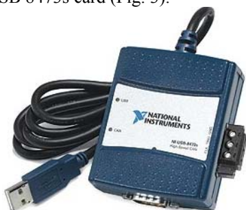
Fig. 3. CAN Highspeed card, NI USB-8473s
