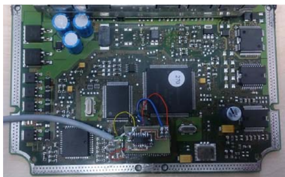
Fig. 12. Modified ECU main board
