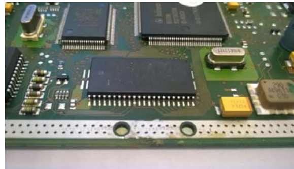
Fig. 1. AM29F512 Flash memory on the motherboard of the engine controller
